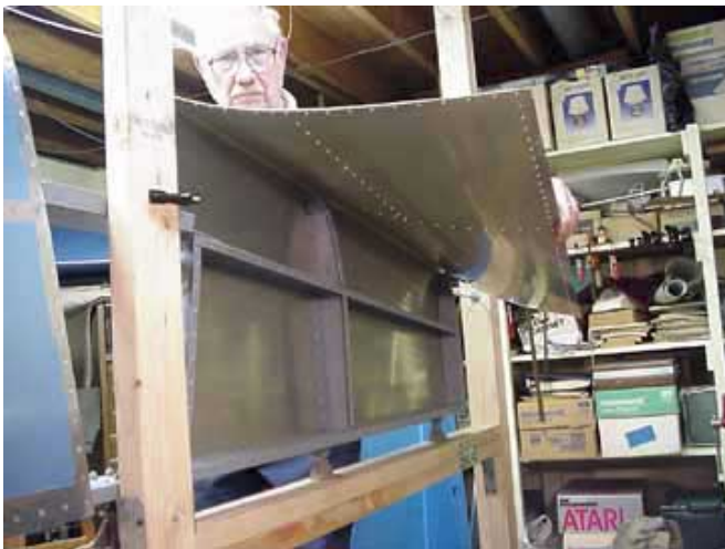
Tom shows the inside riveting pattern for the right horizontal stabilizer.
