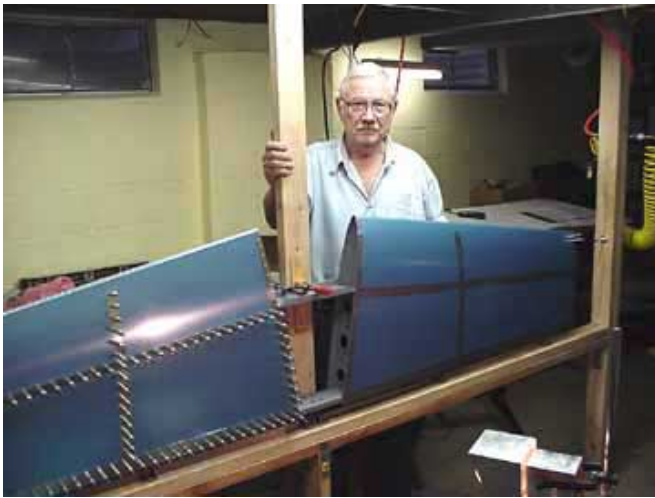
Tom Webster says working on his RV-7A's empennage takes time and patience. Tom and his son Tom Jr. are building the plane in Tom's basement.
