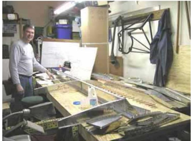
*Bruce Butts reports good progress on his Tailwind. He has acquired the engine mount and landing gear. He is making more ribs, using EAA9's foot metal shear to cut aluminum. The shear is stored at Clare Lutton's shop.*
