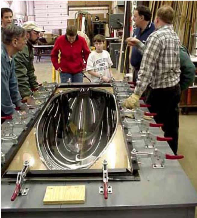
EAA9 members actually helped form a canopy during their visit to Airplane Plastics. Once the plastic is heated, it is placed in a vacuum form which draws down the plastic to a specified shape.
