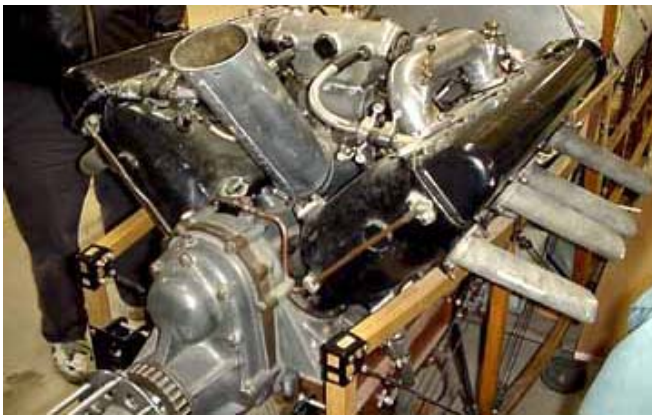
The J-1 is powered by a 180hp V-8 Hispano-Suiza. 1,600 of these units were built.
