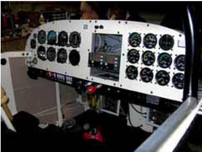
*Tom Webster, Jr., designed and built the RV7A's instrument panel using a computer graphic program to create the template for the panel face. The metal was cut with a high pressure water drill. The windshield has been on, but has been removed to make further accessory installations.*
