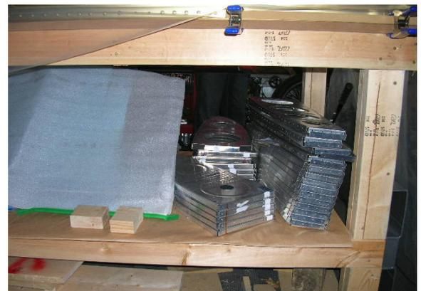
**Wing ribs and parts awaiting completion
