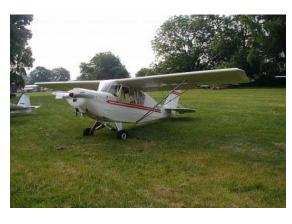
After **Greg Pfeil** made the initial test flight that included stalls, "A few shortcomings were noted." Dave said. "The vertical fin had to be moved 3/8" to the right and the ailerons needed adjustments " He had already incorporated a controllable trim tab in the left elevator, and now he added an aluminum tab to the right side.
